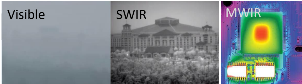
Comparison of visible imagery (left) of a landscape by haze with clear SWIR imagery (right). FPA's and SWIR cameras can see through rain, mist and fog.
